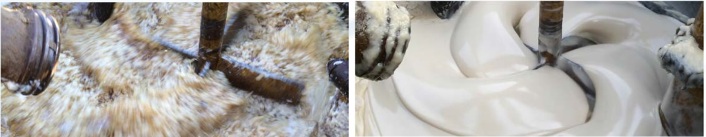
Figure 2: A batch mixer is used to create a fine PARALAX® treated oil for treatment
