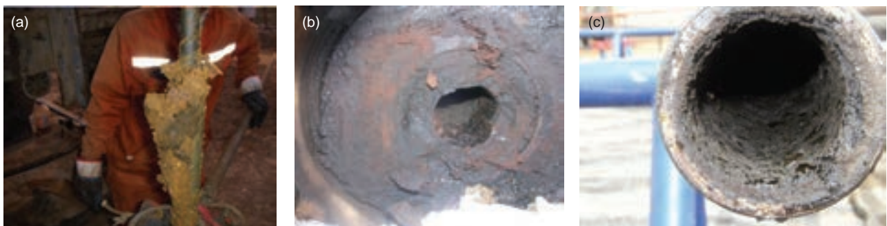
Fig. 1—The effect of wax deposition is shown on (a) a well tubing string, (b) a cross-section of a flowline, and (c) the inside of a tubular. Photos courtesy of OIL CONTROL.
