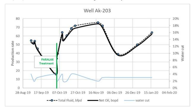
This well was chosen for PARALAX treatment because of sudden drop in production although it was producing fairly low water oil. After the treatment the well so far shows production going up.
