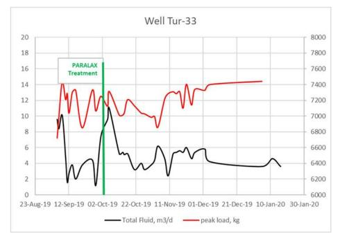
There is an obvious correlation between rod loads and production rate, which is fluid loading.
