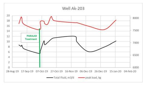
There is an obvious correlation between rod loads and production rate, which is fluid loading.
